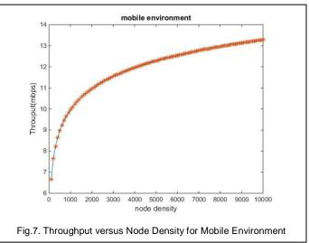
The above graph shows the throughput enhancement in mobile environment with respect to the node density. It can be observed that the throughput has increased nearly 20% as compared with the original in case of mobile network due to effective cross layer approach with cooperative diversity in DEL-CMAC protocol. But it can be observed that in case of static environment the throughput was double than that of mobile environment.
