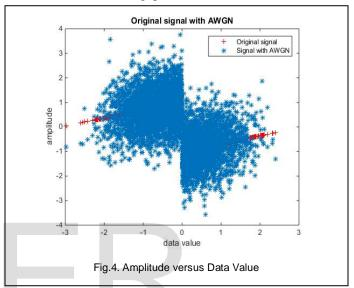
The above graph is plotted between the data value and amplitude. This graph shows the noise (AWGN- Additional White Gaussian Noise) added to the signal while transmitting. While transmitting, if the noise of signal is greater than the threshold value then direct transmission will consume more power and thus decreasing the network lifetime of MANET. In this case cooperative transmission takes place where relay nodes help in transmitting the signal to the destination.
