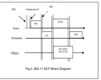
In DCF, after a transmitting terminal senses an idle channel for duration of Distributed Inter Frame Space (DIFS), it backs off for a time period that is chosen from 0 to its Contention Window (CW). After the back off timer expires, the well-known
