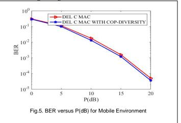
This graph shows the power consumption in both DEL-CMAC with cooperative diversity approach and DEL-CMAC without cooperative diversity. The graph is plotted for Bit-Error-Rate versus Power measured in dB. The above graph shows that
