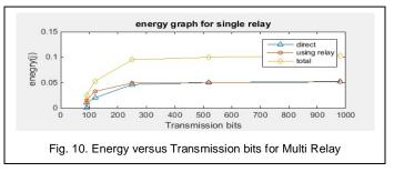
The above graph shows the energy consumption for multiple relays in mobile environment.
